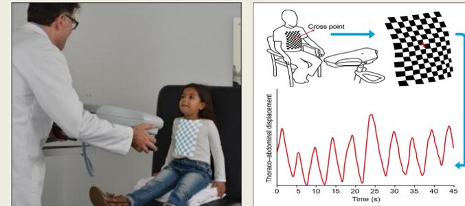
Figure 1: Structured Light projected onto the thoraco-abdominal (TA) wall of a participant seated approximately 1 meter from the device (Thora-3DITM, PneumaCare, Cambridge, UK).
